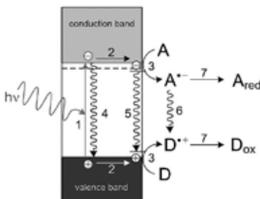
Primary physical and chemical processes occurring in the presence of irradiated photocatalyst.
