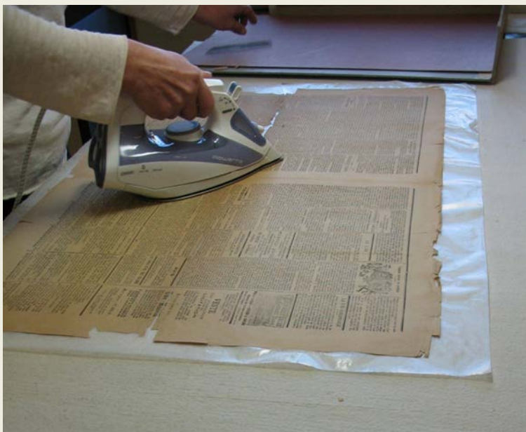
Complete lining of a very brittle sheet
