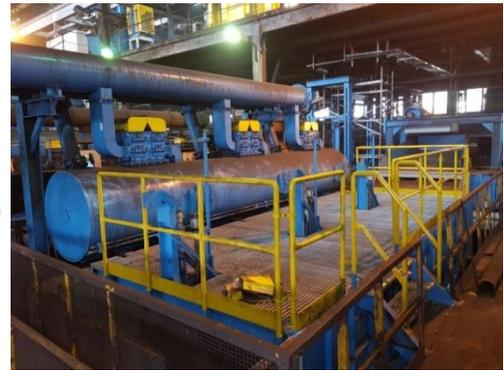
**Fig. 20.** OM 20 fines jig [KOMAG]
