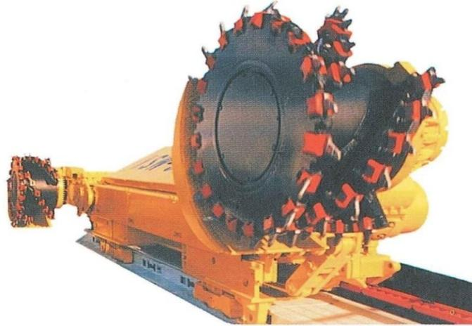
**Fig. 14.** KSE-500 longwall shearer [KOMAG]
