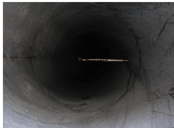
**Fig. 2b.** Measuring probe with the filter installed in the tested venturi pipeline
