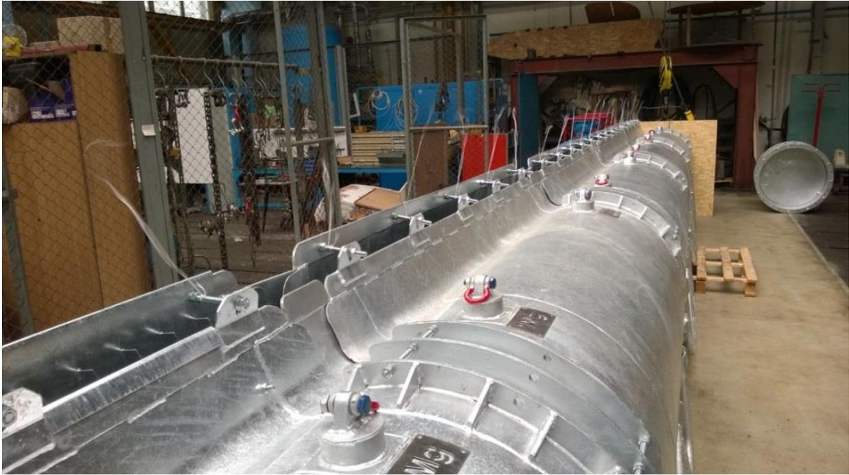
Fig. 6. Correctly adjusted vortex ventube
