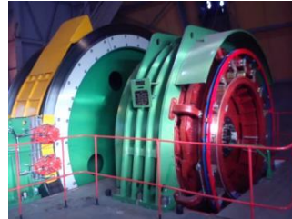
Fig. 2. Two-rope hoisting machine of Koepe type
