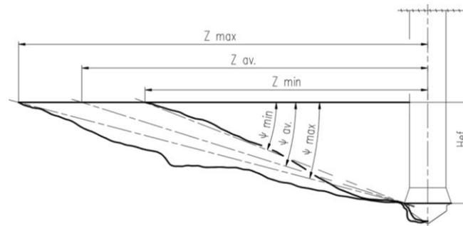
**Fig. 18.** Cross-section through the loosened solid and the method for determination of the effective anchoring depth  $H_{ef}$ , maximum, minimum and average range  $Z_{max, min, av}$  as well as loosening angle  $\psi_{max, min, av}$  [34]
