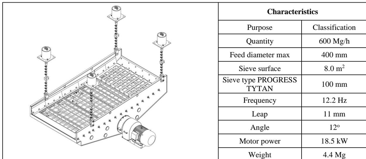
Fig. 2. WK1-2.0x4.0 vibrating screen
