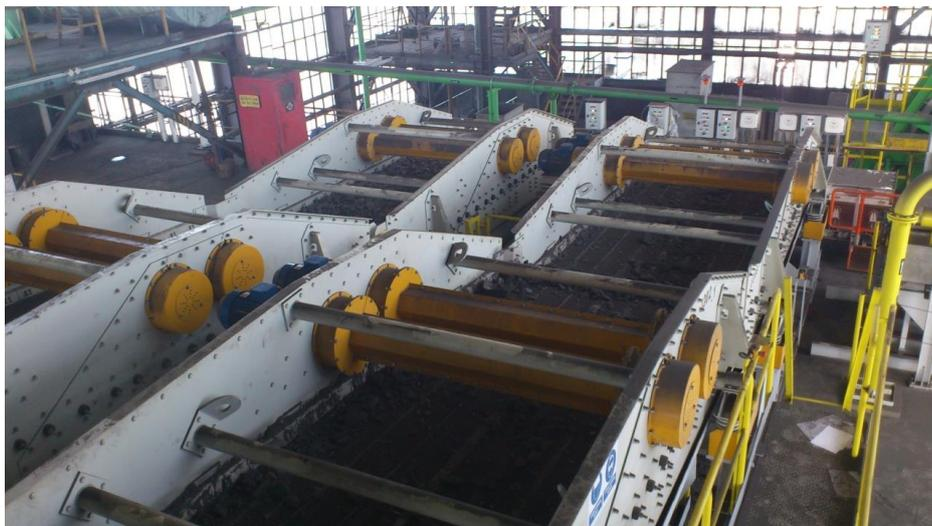
Fig. 5. Two tandem vibrating screens PWP1-2.2x5.25
