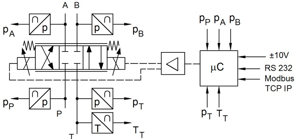
**Fig. 1.** Simplified scheme of proportional directional valve with intelligent module
