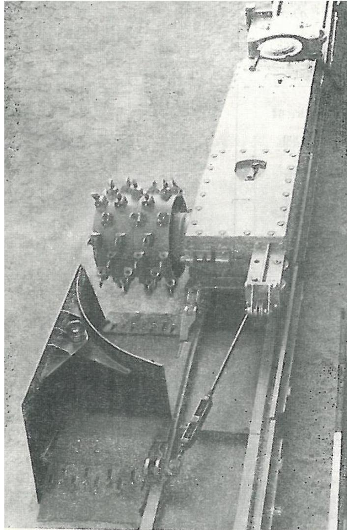
**Fig. 5.** First Polish single drum shearer with rope haulage system with parabolic drive wheel. [14]
