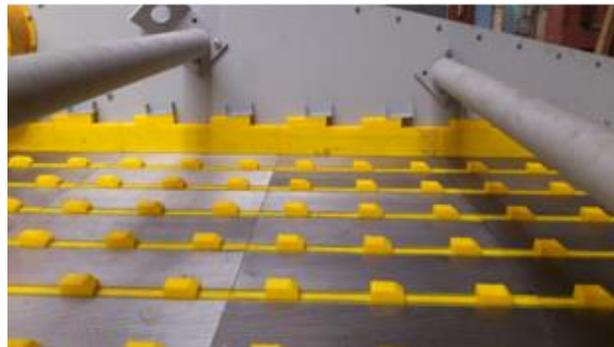
**Fig. 14.** Sieve deck, slotted, welded, built-in PRO-CLIN system
