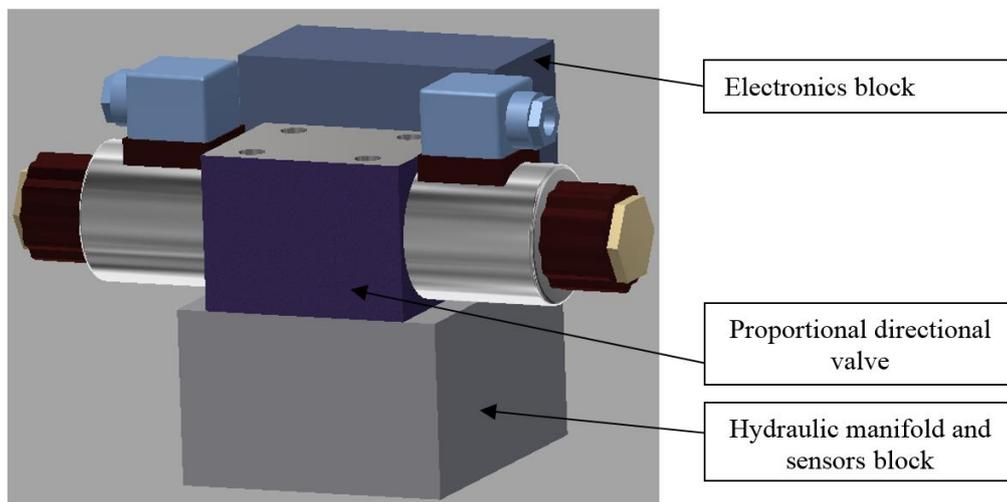
**Fig. 2.** Proposed constructive form of the intelligent module for proportional directional valve
