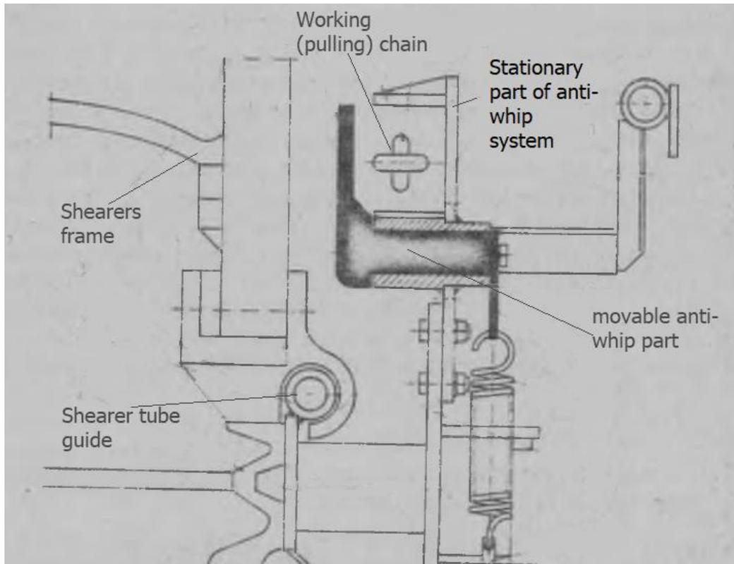
**Fig. 9.** Example of working chain anti-whip grip system [19]
