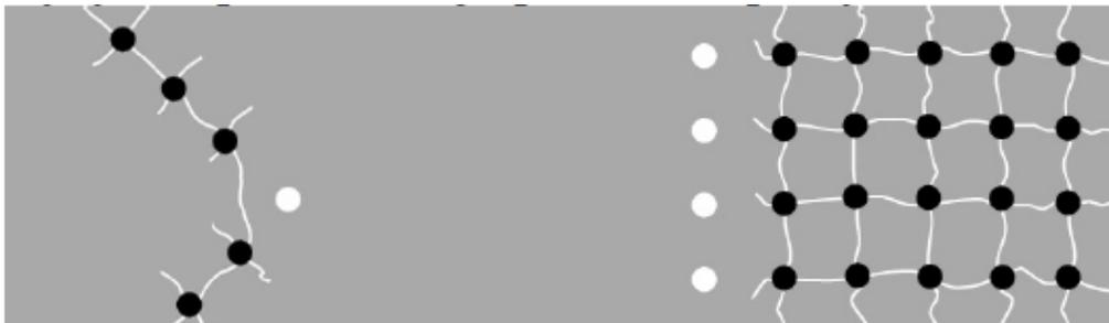
**Fig. 10.** Directions of cracks propagation in the rock block depending on the place of using the expanding materials [22]
