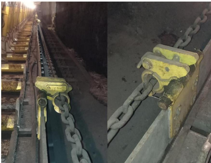
**Fig. 8.** Simply, hand operated anti-whip grips in longwall face [author's]
