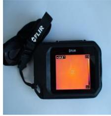
**Fig. 24.** Pocket model FLIR camera
