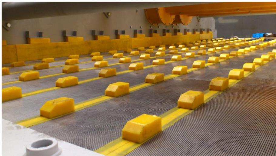
Fig. 9. Installation of deck in the PWP1-2.4x5.25 screen
