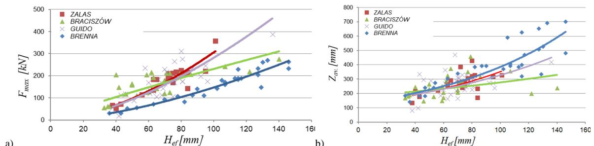
**Fig. 19.** Functions of the effective anchoring depth: a) loosening force  $F_{max}$  and b) average destruction ranges  $Z_{av}$ , depending on effective anchoring depth  $H_{ef}$  for different rock types [33]
