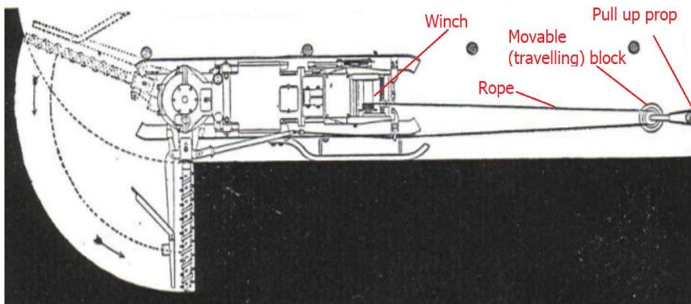
**Fig. 3.** First free rope haulage system with winch [12]
