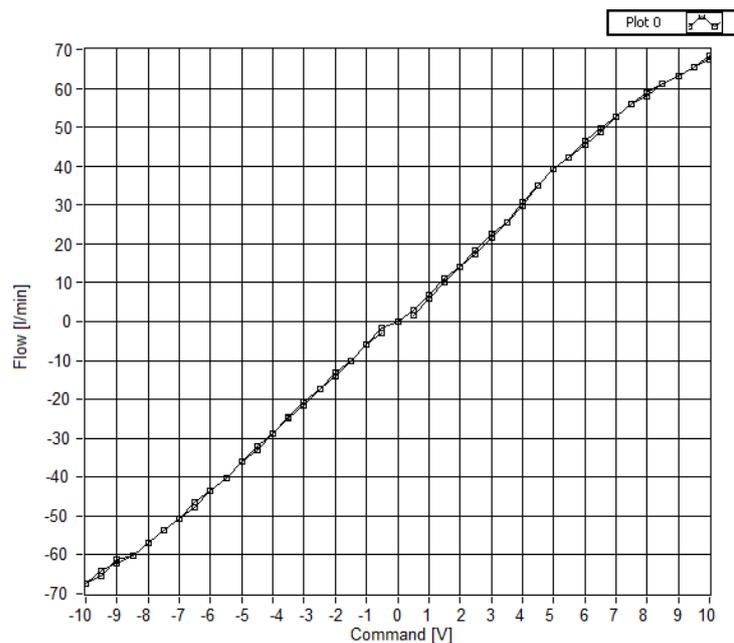
Fig. 8. Static characteristic for a proportional directional valve
