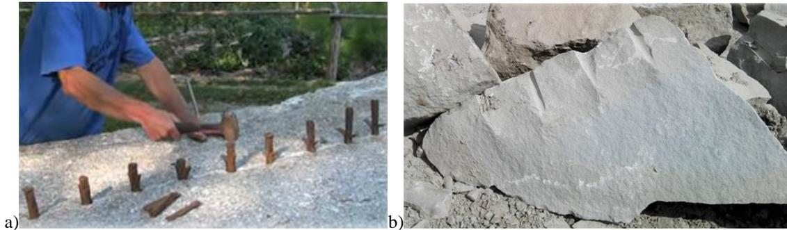
**Fig. 7.** An example of manual mechanical wedging: a) process in progress [19], b) the fracture plane of the rock block after using this method [20]
