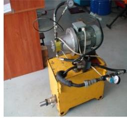
**Fig. 25.** Testing stand for gear pumps
