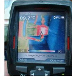
**Fig. 27.** Defective working pump
