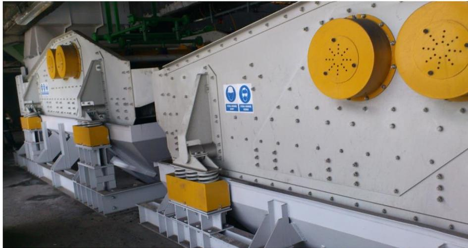
**Fig. 11.** DISA concentrator coal output, feed to dewatering and sorting sieve
