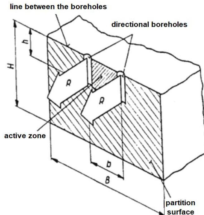
**Fig. 6.** Diagram of the conditions of rock separation by the spreading method;
