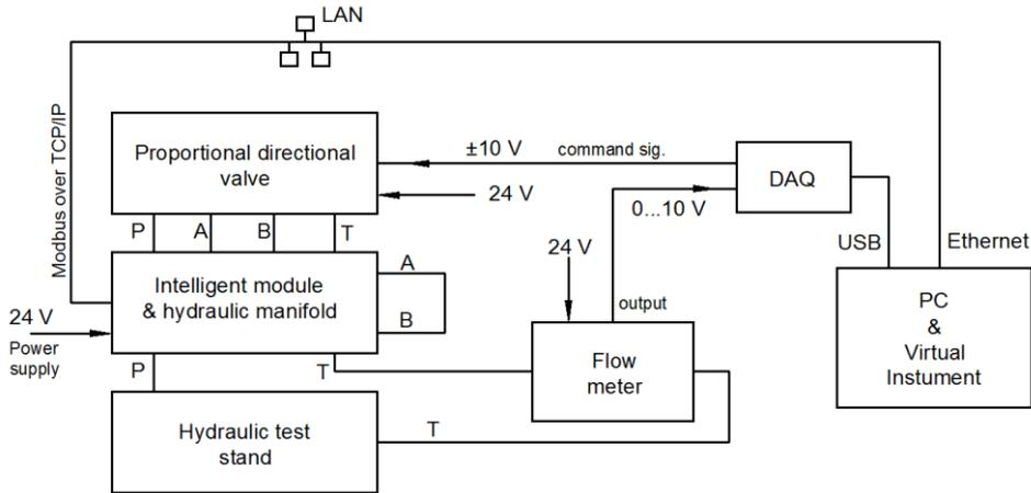
Fig. 5. Block diagram with data acquisition system
