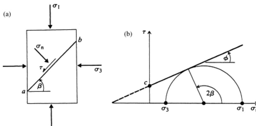
Fig. 5. Graphical interpretation of the rock sample failure surface after the test of three-axial compression for  $\sigma_1 \neq \sigma_3$  and  $\sigma_1 > \sigma_3$  and  $\sigma_2 = \sigma_3$  for Coulomb – Mohr criterion [16]
