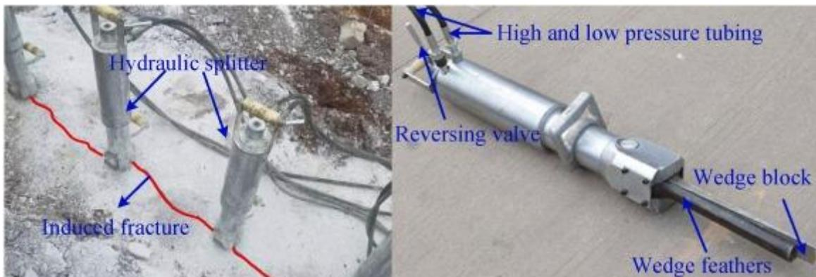
**Fig. 8.** Hydraulic splitter employed for the non-explosive fracturing of rock in engineering application [21]
