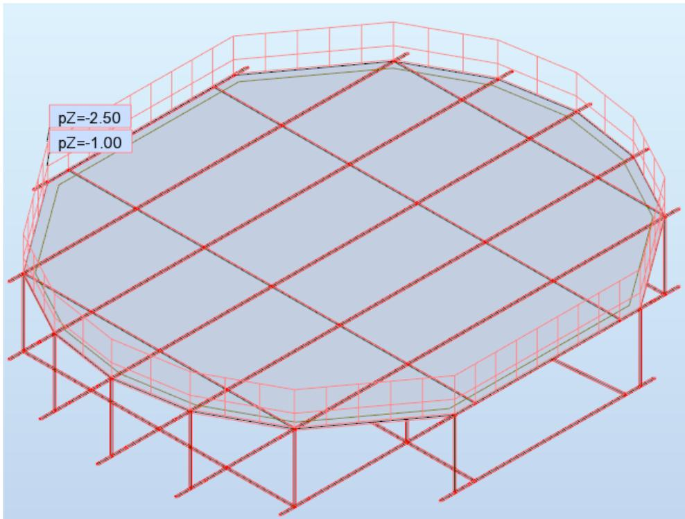
Fig. 6. Forces acting on the model (units:  $\text{kN/m}^2$ )
