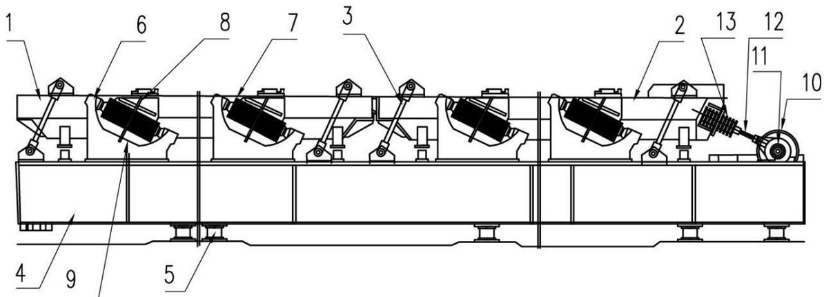
**Fig. 4.** GRO-1 triple-mass resonance screen
