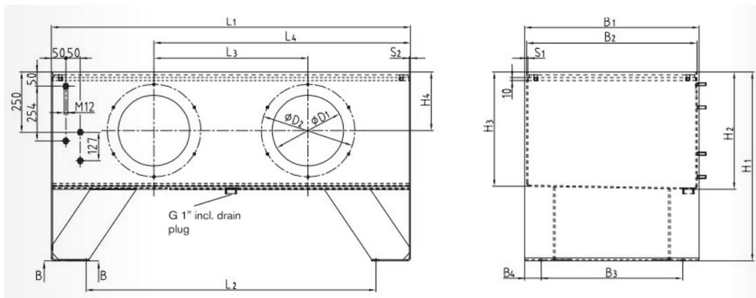
Fig. 6. Sample tank for a coolant [17]
