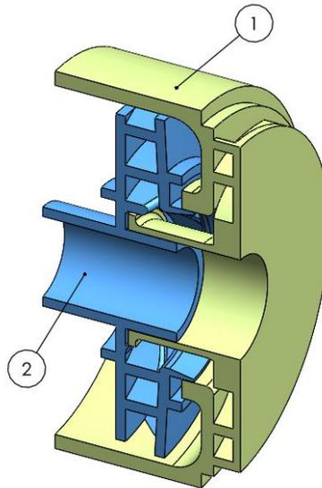
**Fig. 5.** A three-dimensional model of a submersible centrifugal pump section
