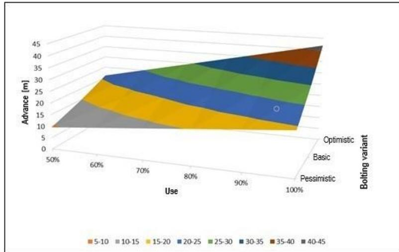
Fig. 6. Relationship between advance and bolting variant
