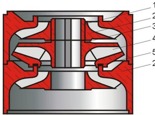
**Fig. 3.** Stage of a submersible pump
