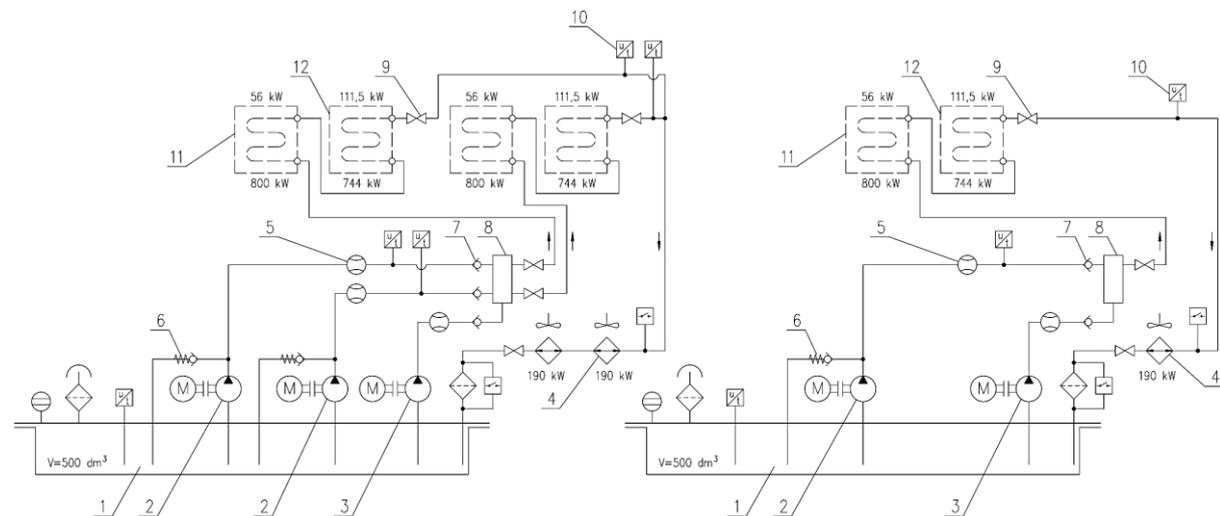
**Fig. 8.** Diagram of the underground cooling system of conveyor belt drives: 1 - tank, 2, 3 - pump units, 4 - air-water cooler, 5 - flow meter, 6, 7 - check valves, 8 - collector, 9 - cut-off valve, 10 - temperature sensor, 11 - electric motor flow system, 12 - gear flow system
