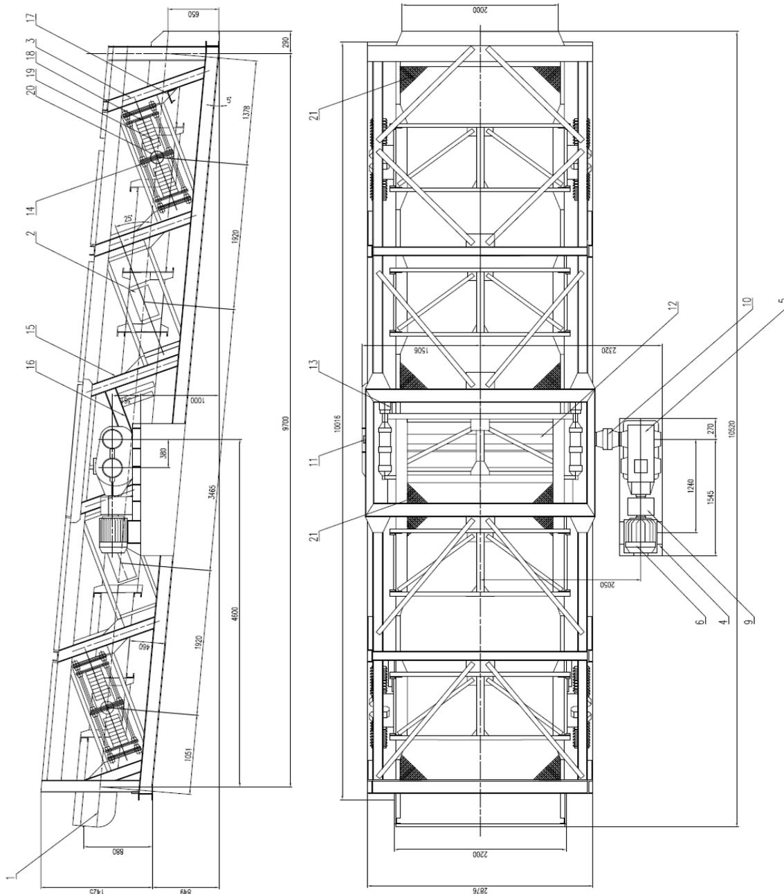
Fig. 8. Preliminary design of the 85K resonance screen [21]
