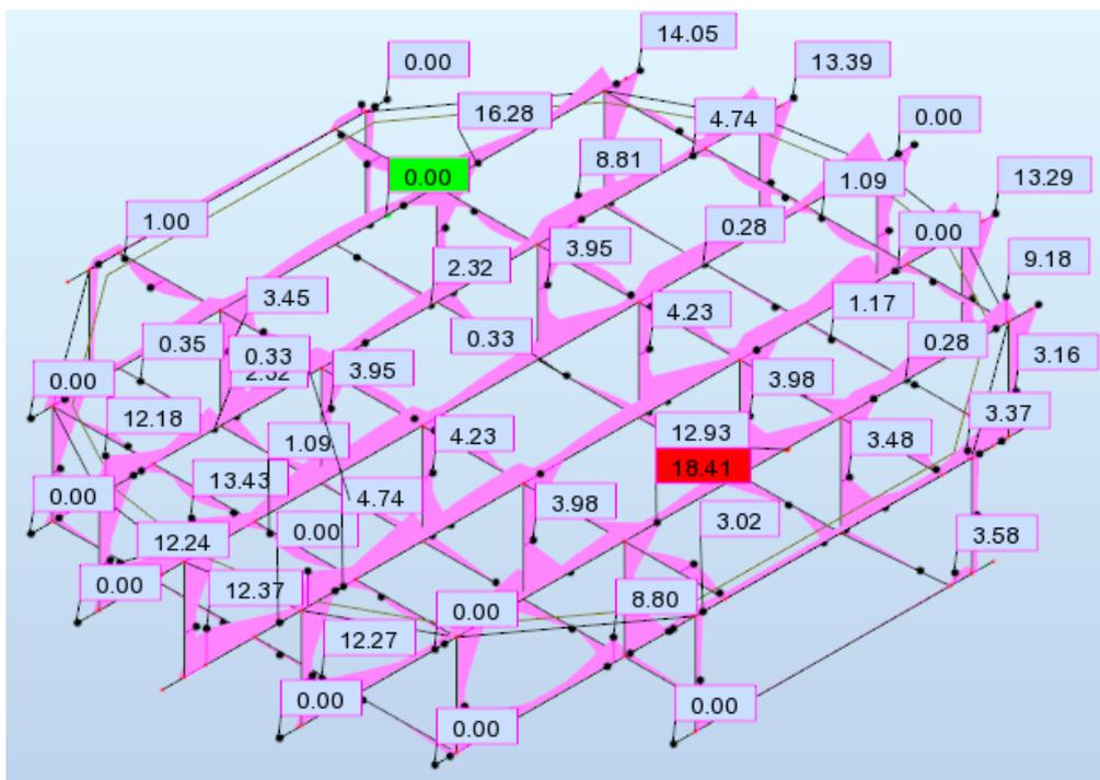
Fig. 7. Values of stress calculated (units: MPa)
