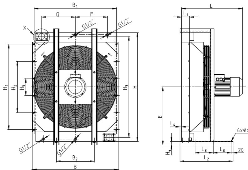
**Fig. 4.** View of the cooler for use in a potentially explosive atmosphere [16]
