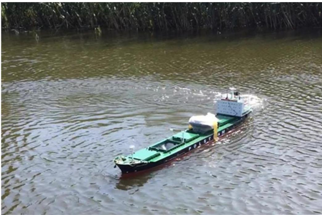
Fig. 6 Ship's model during circulation investigations [4,11]
